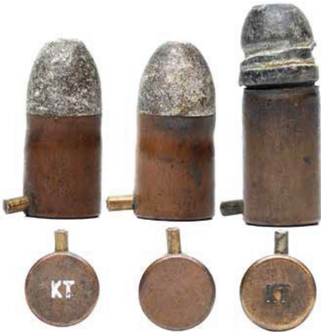
The above three are Danish military cartridges made at Københavns Tøjhus . In English this would be "Copenhagen Arsenal." These first two were made for their pinfire revolvers that they named as Danish M/1861, M/1865 and M/1871 revolvers. It is unknown what specific gun the carbine-length cartridge was made for.
